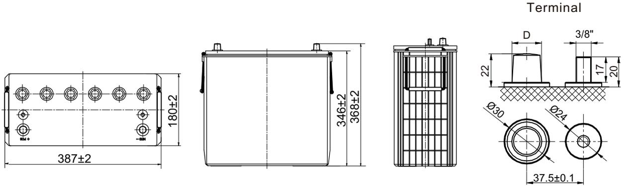
Note: D: Positive 19.5<sup>0</sup><sub>-0.3</sub>; D: Negative 17.9<sup>0</sup><sub>-0.3</sub>; Terminal Torque Values in-lb(Nm): 176-203(20-23)
