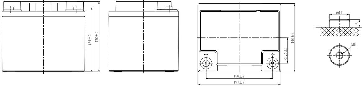
Note: Terminal Torque Values in-lb(Nm):34.39-47.75(3.9-5.4)
